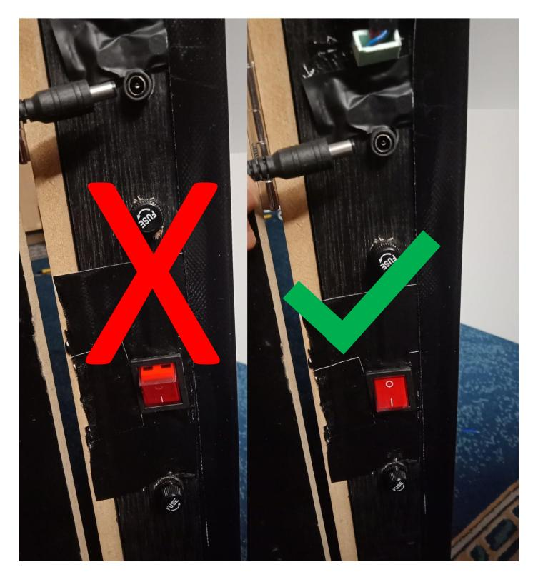
Turn off the switch first and plug out the power cable.
